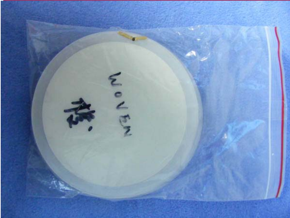
TWO PHOTOGRAPHIC STANDARDS INSIDE ONE FOR WOVEN FABIC ANOTHER FOR KNITTED FABRIC
